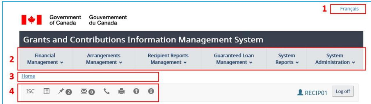
The GCIMS screen consists of four (4) navigational sections that are displayed the entire time that you are logged on to GCIMS:
